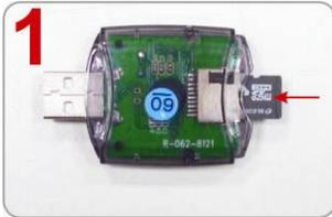
Insert the SD card into the card reader (Please make sure the direction is correct)
