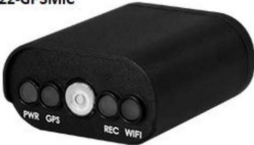
The optional EX22-GPSMIC is a multi-function device that can be added to the system.
